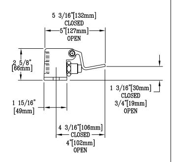
NOTE 1. INLETS & OUTLET ARE 1/2" NPT FEMALE NOTE 2. FURNISHED WITH (2) WOOD MOUNTING SCREWS
