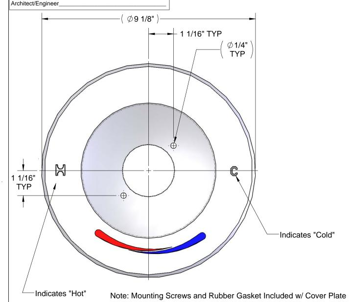
Drawn Checked Approved Product Specifications: ARH DMH JHB **Cover Plate** for Pressure Balance Valve, Date: Scale: B-3204 1:2 11/05/08
