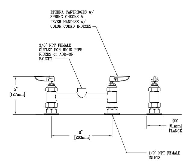
NOTE: RIGID BASE MAY BE CONVERTED TO SWIVEL BY SPECIFYING B-0412 RIGID to SWIVEL ADAPTER.
