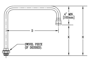
SPECIFY D, H, & K DIMENSIONS REQUIRED AND IF GOOSENECK IS TO BE RIGID OR SWIVEL.
