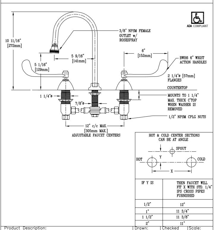
12" c/c DECK MOUNTED MIXING FAUCET w/ 6" WRIST ACTION HANDLES, ADJUSTABLE INLET CENTERS, AND RIGID GOOSENECK w/ ROSESPRAY OUTLET
