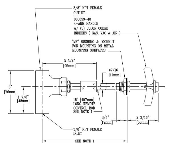
NOTES: 1. STANDARD ROD LENGTH IS 18". WHEN ORDERING, SPECIFY ACTUAL LENGTH DESIRED. MINIMUM IS 4 1/2" [114mm]
