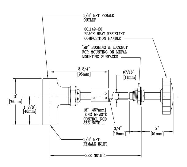
NOTES: 1. STANDARD ROD LENGTH IS 18". WHEN ORDERING, SPECIFY ACTUAL LENGTH DESIRED. MINIMUM IS 4 1/2" [114mm]
