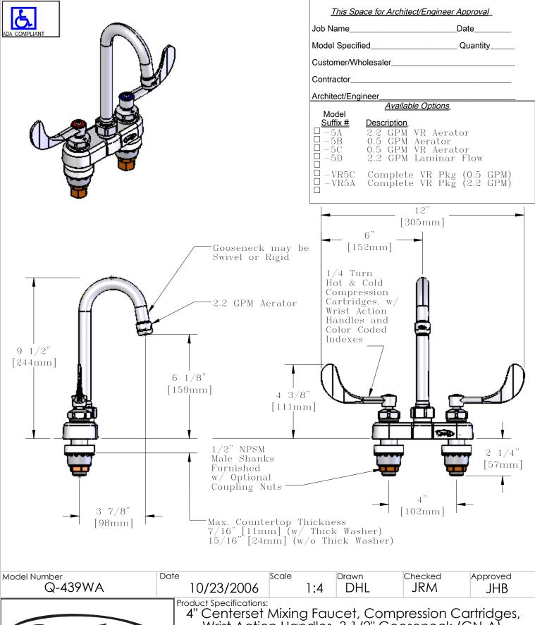
4" Centerset Mixing Faucet, Compression Cartridges, Wrist Action Handles, 3 1/2" Gooseneck (GN-A), 2.2 GPM Aerator
