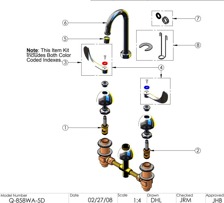
Product Specifications: 8" Widespread Mixing Faucet, Ceramic Cartridges, Wrist Action Handles, 3 1/2" Gooseneck (GN-A) & 2.2 GPM Laminar Device
