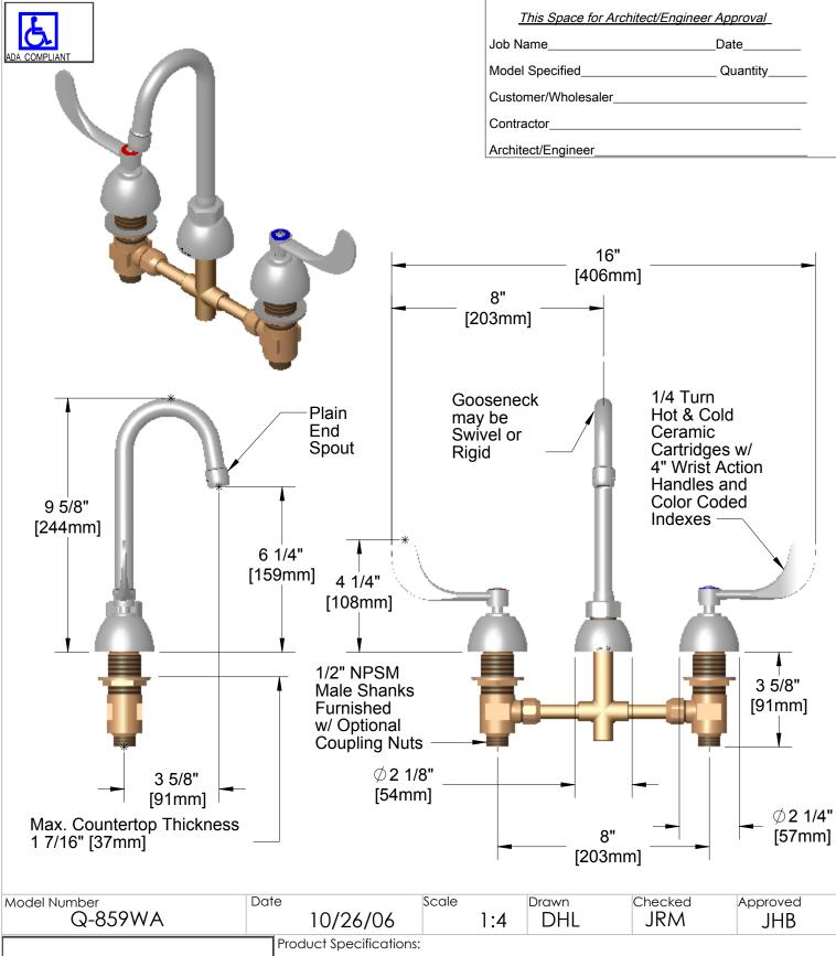
8" Widespread Mixing Faucet, Compression Cartridges, Wrist Action Handles, 3 1/2" Gooseneck (GN-A)
