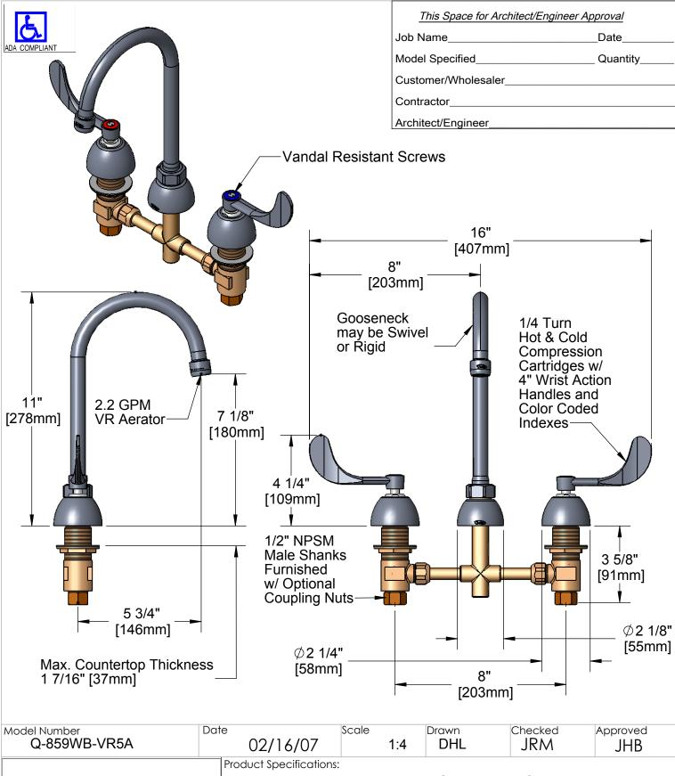
8" Widespread Mixing Faucet, Compression Cartridges, Wrist Action Handles w/ Vandal Resistant Screws, 5 3/4" Gooseneck (GN-B), 2.2 GPM Vandal Resistant Aerator
