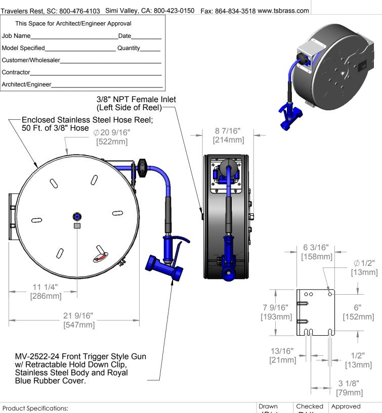
3/8" x 50 Ft. Enclosed Stainless Steel Reel MV-2522-24 Front Trigger, 5/16" Spray Gun
