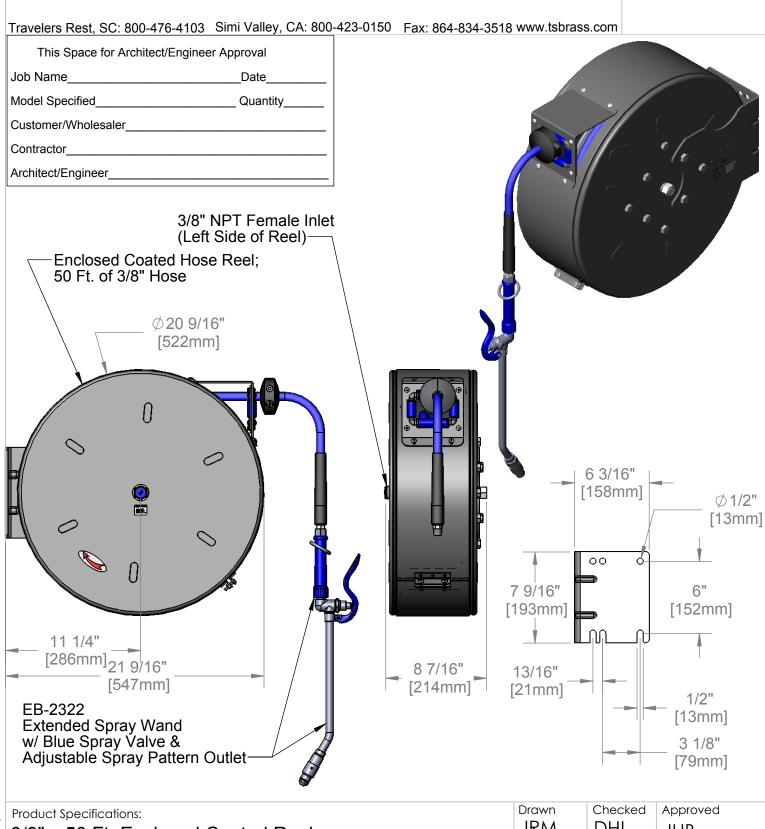
3/8" x 50 Ft. Enclosed Coated Reel w/ EB-2322 Extended Spray Wand w/ Blue Spray Valve
