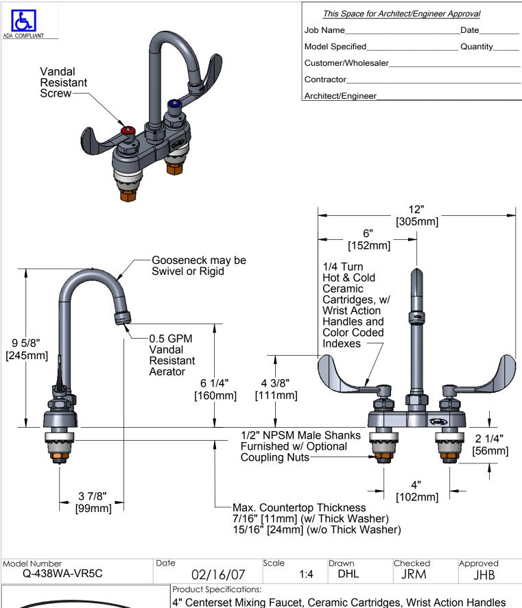
w/ Vandal Resistant Screws, 3 1/2" Gooseneck (GN-A), 0.5 GPM Vandal **Resistant Aerator**
