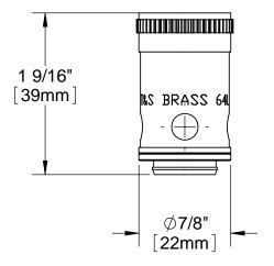
Drawn Checked Approved **Product Specifications: ARH GEF JHB** Right Hand (Hot) Cartridge Barrel Date: Scale: 1:1 11/11/08
