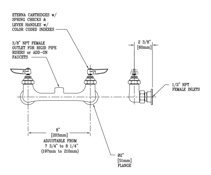
NOTE: RIGID BASE MAY BE CONVERTED TO SWIVEL BY SPECIFYING B-0412 RIGID to SWIVEL ADAPTER.
