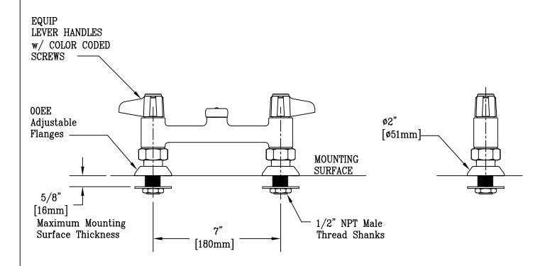
NOTE: ROUGH-IN REQUIREMENTS Ø1 1/4" [Ø32mm] HOLES Ø1" [Ø25mm] Minimum
