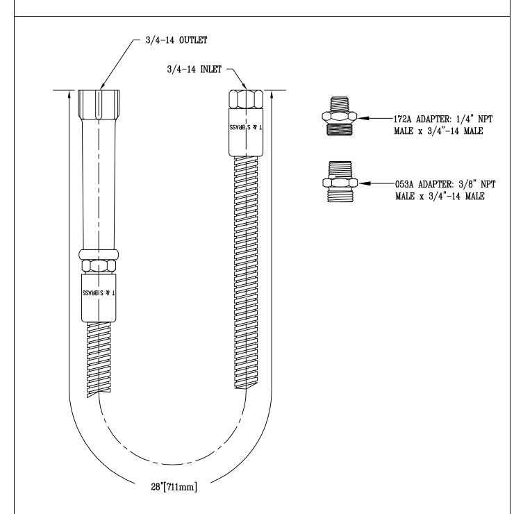
28" FLEXIBLE ST. STEEL HOSE ASM. WITH 172A & 053A ADAPTERS
