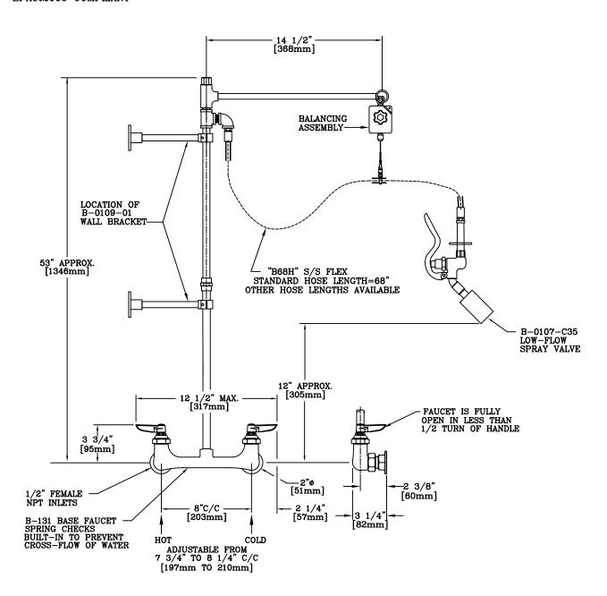
NOTE: ALSO AVAILABLE WITH 1/2" NPT MALE INLETS AND LOCKNUTS ON FAUCETS IN PLACE OF FEMALE INLETS.
