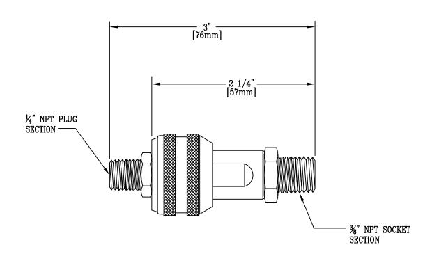
FOR USE WITH WATER, AIR, AND NON-CORROSIVE GASES.
