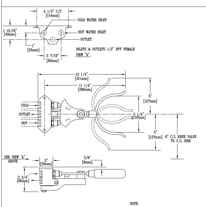
FURNISHED WITH 1/4"-20 SCREWS & NUTS FOR MOUNTING ON CHAIR CARRIER CROSS BAR
