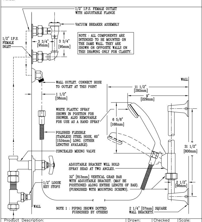
PATIENT'S BATH FITTING WITH CONCEALED MIXING VALVE. LOOSE KEY STOPS, VACUUM BREAKER, WALL OUTLET, STAINLESS STEEL HOSE, & GRAB BAR W/ ADJ. BRACKET
