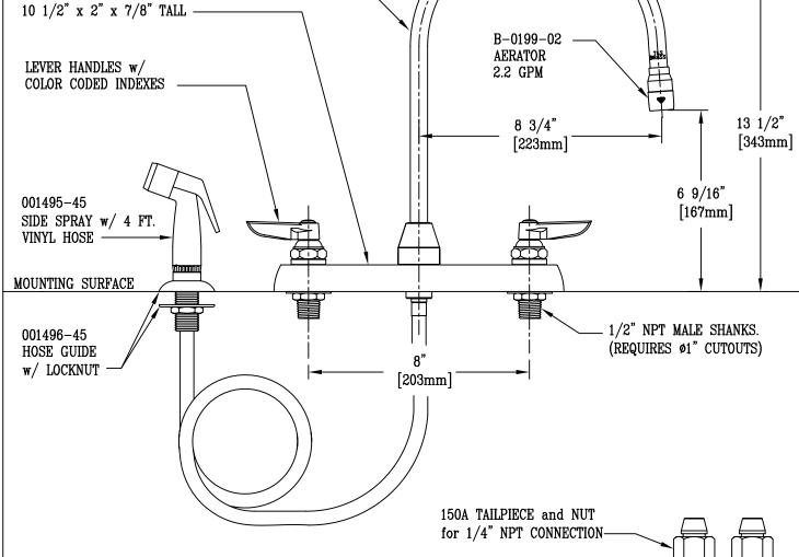
Product Description: WORKBOARD FAUCET w/ 1/2" NPT MALE SHANKS, 8" INLET CENTERS, SWIVEL GOOSENECK ASM, SIDE SPRAY w/ HOSE, B-0199-02 AERATOR & LEVER HANDLES
