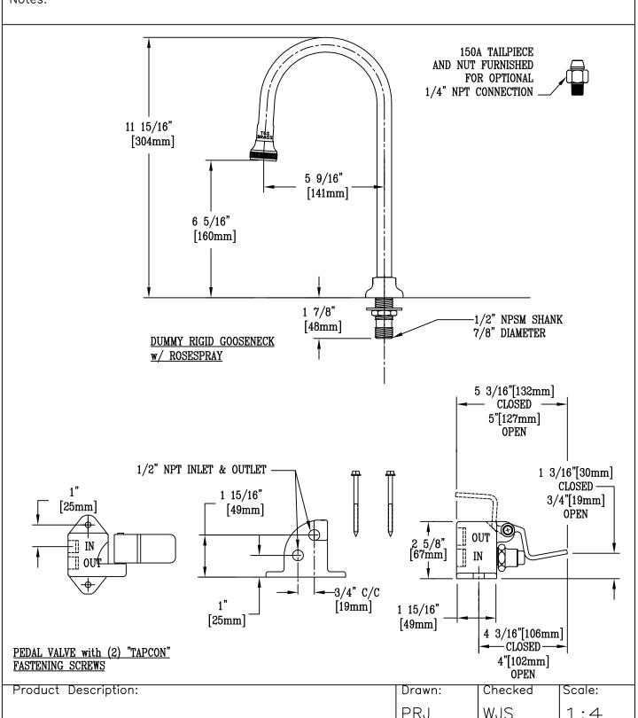
B-0507 SINGLE PEDAL VALVE w/ B-0524 RIGID DUMMY
