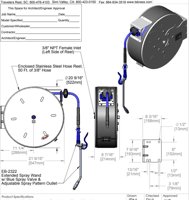
3/8" x 50 Ft. Enclosed Stainless Steel Reel w/ EB-2322 Extended Spray Wand & Blue Spray Valve
