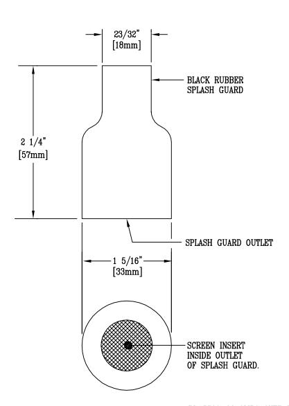
BL-5500-02 SLIPS OVER THE OUTLET OF MODEL NO. BL-5500-0 FILTER PUMP TO ELIMINATE SPLASH.
