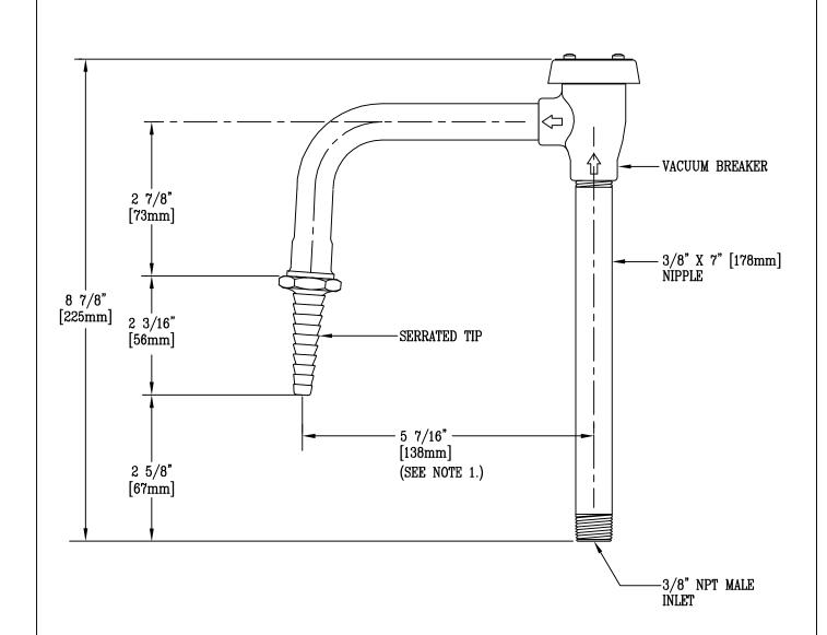
NOTE: NOZZLE IS AVAILABLE WITH 4"[102mm], 9"[229mm], OR 12" [305mm] SPREAD WHEN SPECIFIED.
