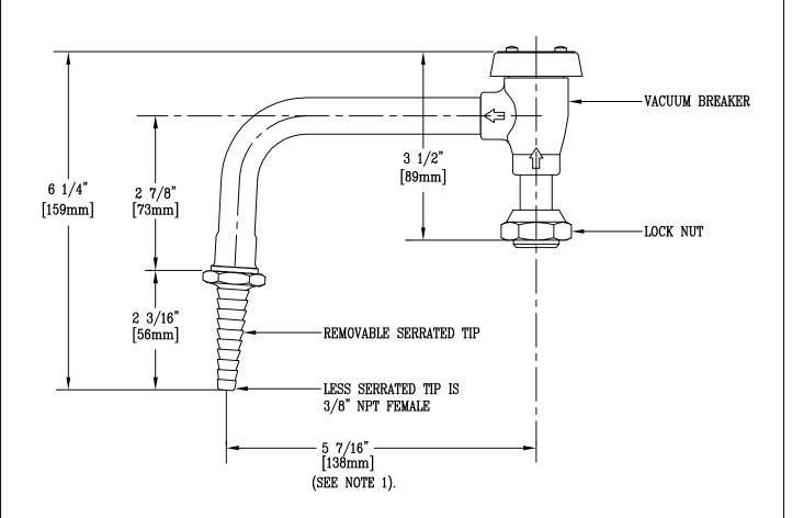
NOTE: NOZZLE IS AVAILABLE WITH 4"[102mm], 9"[229mm], OR 12" [305mm] SPREAD WHEN SPECIFIED.
