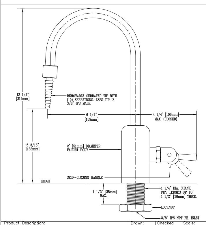
GRAY PVC SINGLE LEDGE FAUCET WITH RIGID GOOSENECK & SERRATED TIP FOR DISTILLED WATER, WITH SELF—CLOSING OPERATION
