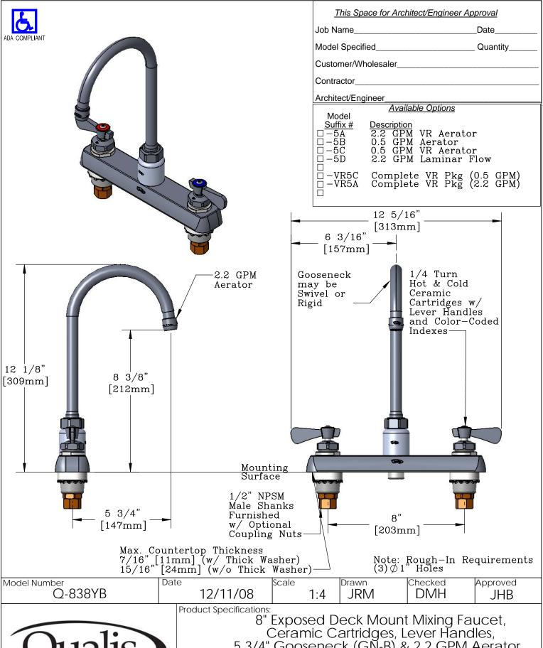
5 3/4" Gooseneck (GN-B) & 2.2 GPM Aerator
