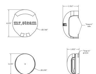
**IMPORTANT NOTE:** Install steamhead with acrylic shield according to orientation illustrated above. Steam vents out of steam slots to left and right of steamhead. Refer to Installation and Operation Manual, PUR 100376, for complete installation details.
