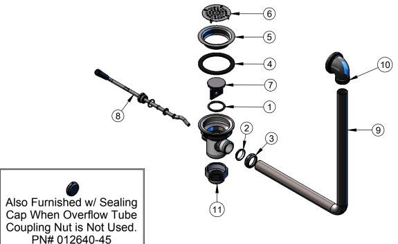
Rotary Waste Valve w/ Twist Handle, 3 1/2" Sink Opening, 2" NPT Female x 1 1/2" BSP Male Adapter & Overflow Tube w/ Head Asm.
