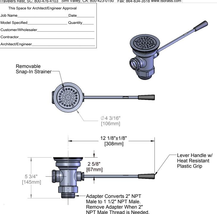
Waste Drain Valve w/ Lever Handle, 3" Sink Opening, 2" NPT Male Outlet & 1 1/2" NPT Male Adapter
