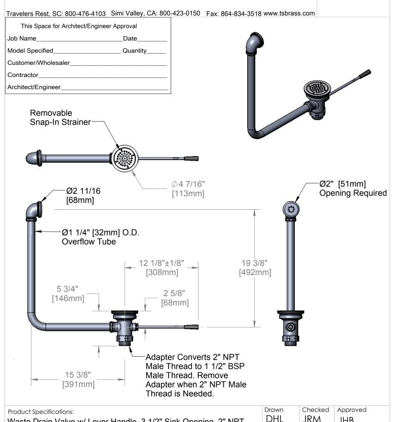
Waste Drain Valve w/ Lever Handle, 3 1/2" Sink Opening, 2" NPT Female x 1-1/2" BSP Male Adapter & Overflow Tube w/ Head Asm.
