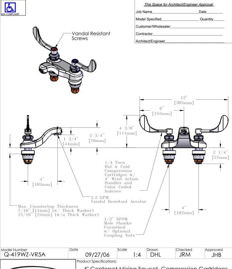
4" Centerset Mixing Faucet, Compression Cartridges, Wrist Action VR Handles, 2.2 GPM VR Aerator
