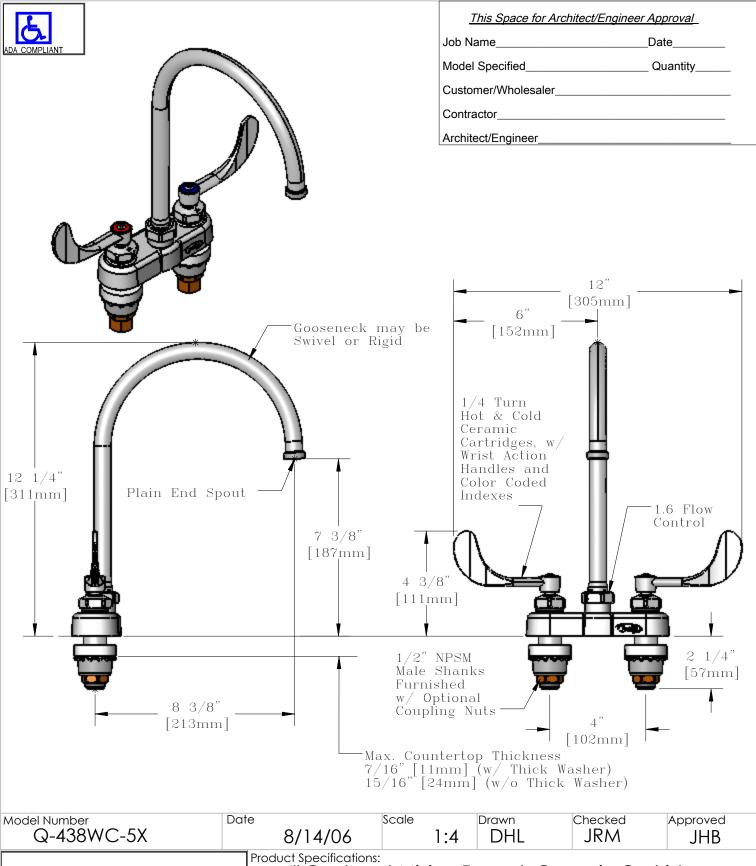
4" Centerset Mixing Faucet, Ceramic Cartridges, Wrist Action Handles, 8" Gooseneck (GN-C), 1.6 GPM Flow Control
