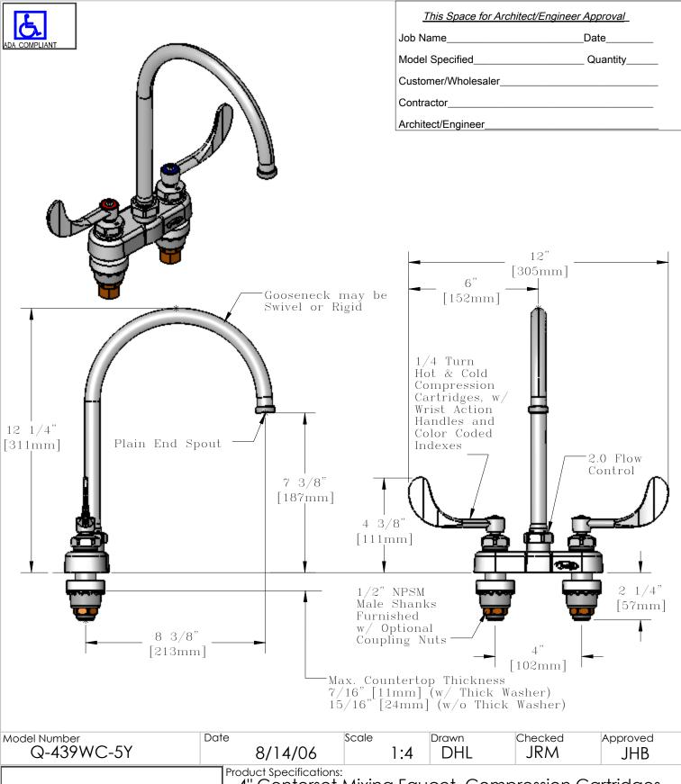
4" Centerset Mixing Faucet, Compression Cartridges, Wrist Action Handles, 8" Gooseneck (GN-C), 2.0 GPM Flow Control
