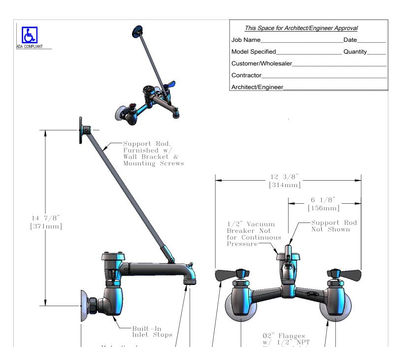
·1/4 Turn Hot & Cold Compression Cartridges w/ Lever Handles and Color Coded Indexes
