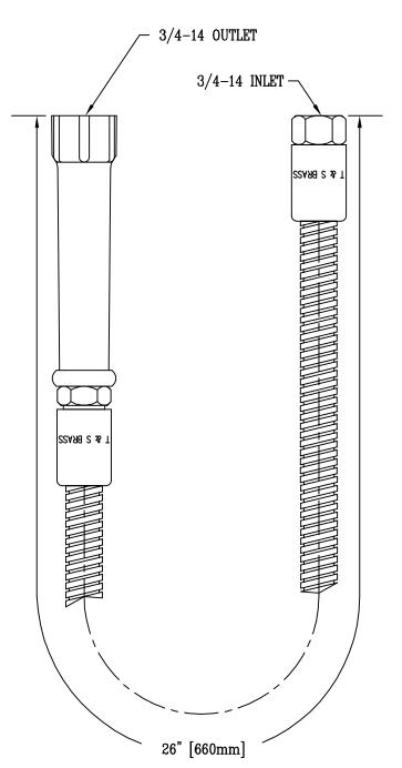
FLEX STAINLESS STEEL HOSE WITH POLYURETHANE INNER HOSE
