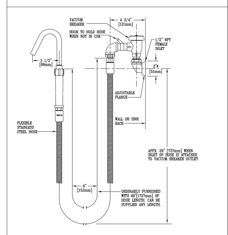
Product Description: KETTLE & POT FILLER ASSEMBLY WITH FLEXIBLE STAINLESS STEEL HOSE, VACUUM BREAKER, AND
