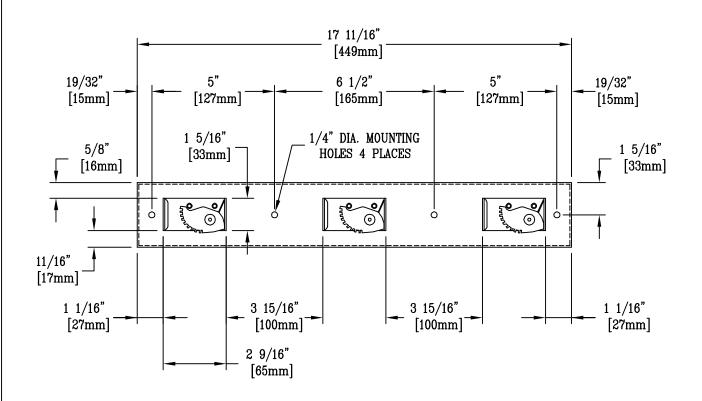
FURNISHED WITH #10 x 1 1/2" WOOD SCREWS AND WALL ANCHORS
