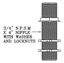
POLISHED ALUMINUM ELECTRICAL BOX SUPPLIED WITH DUPLEX, 3 WIRE RECEPTACLES, COVERPLATE AND SUPPLY NIPPLE WITH LOCKNUTS AND WASHER.
