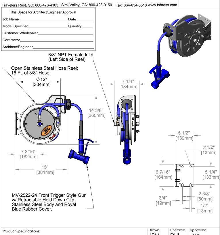
Hose Reel System: 3/8" x 15 Ft. Open Stainless Steel Reel MV-2522-24 Front Trigger, 5/16" Spray Gun
