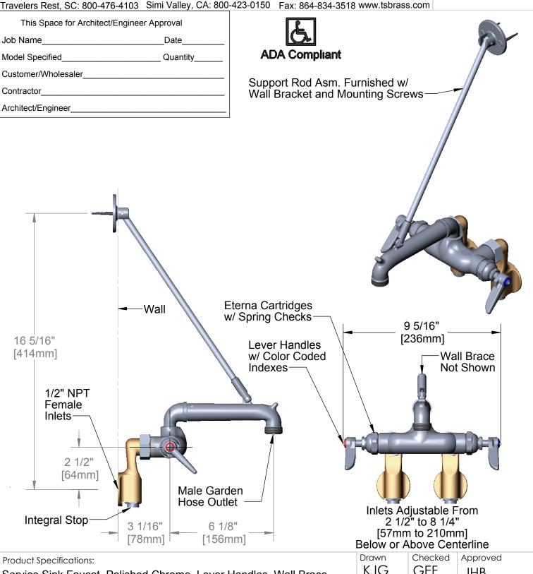
Service Sink Faucet, Polished Chrome, Lever Handles, Wall Brace, 1/2" NPT Adjustable Inlets w/ Integral Stops & Male Garden Hose Outlet
