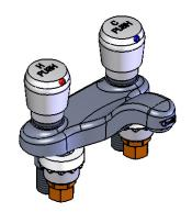
Metering Cartridges, w/ Push Button Handles and Color Coded Indexes 3 1/4" 2 3/4" [86mm] 1 3/4" [70mm] [44mm] 2 1/4" 2.2 GPM VR Aerator 1/2" NPSM Male Shank [102mm] [102mm] Furnished w/ Optional Coupling Nuts Max. Countertop Thickness 7/16" [11mm] (w/ Thick Washer) 15/16" [24mm] (w/o Thick Washer)
