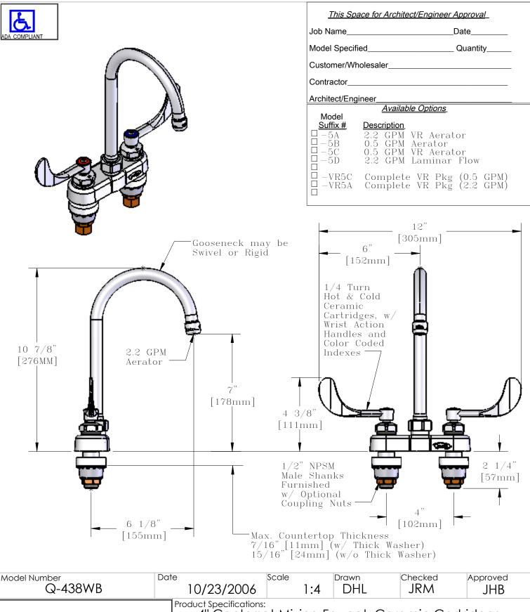
4" Centerset Mixing Faucet, Ceramic Cartridges, Wrist Action Handles, 5 3/4" Gooseneck (GN-B), 2.2 GPM Aerator
