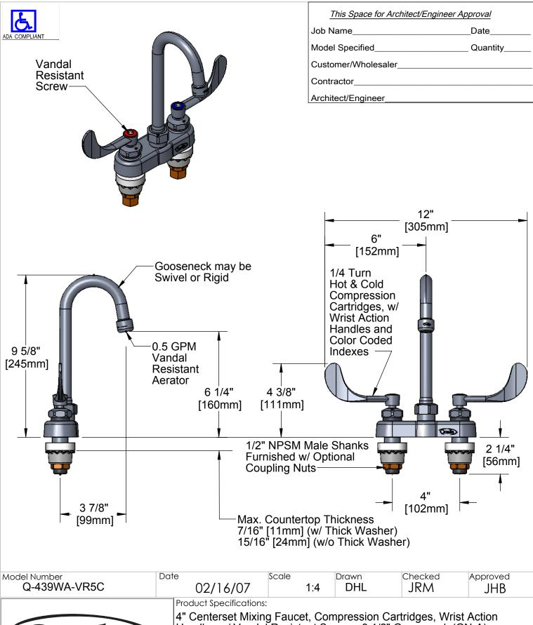
Handles w/ Vandal Resistant Screws, 3 1/2" Gooseneck (GN-A). 0.5 GPM Vandal Resistant Aerator
