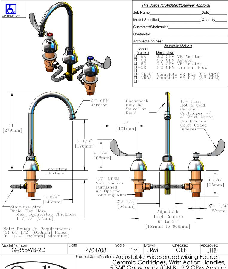
5 3/4" Gooseneck (GN-B), 2.2 GPM Aerator & Flex Lines
