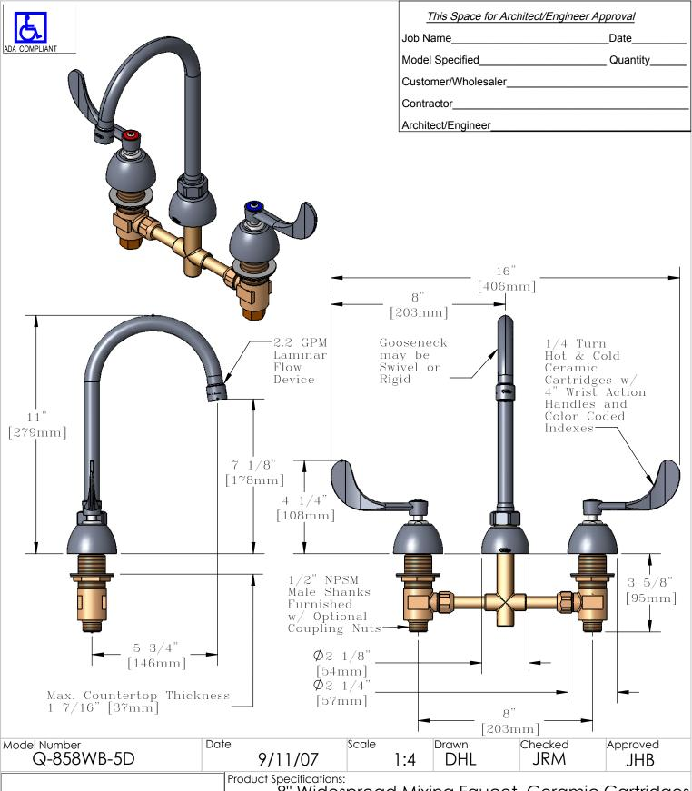
8" Widespread Mixing Faucet, Ceramic Cartridges, Wrist Action Handles, 5 3/4" Gooseneck (GN-B), 2.2 GPM Laminar Flow Device
