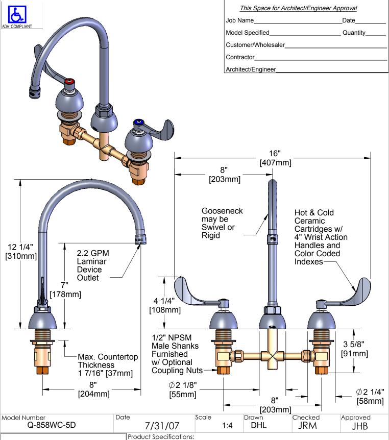
8" Widespread Mixing Faucet, Ceramic Cartridges, Wrist Action Handles, 8" Gooseneck (GN-C), 2.2 GPM Laminar Device Outlet
